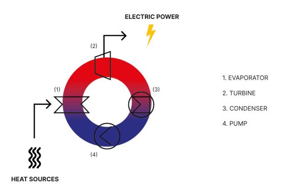
Heat from a heat source evaporates, through an evaporator heat exchanger (1), a low-boiling-point working fluid which expands spinning a turbine (2) attached to an alternator generating electric power. The working fluid is then condensed in a condenser heat exchanger (3) and pumped back (4) to the first exchanger, thus closing the loop. Residual heat from the condenser can also be used as a resource for CHP (Combined Heat & Power generation).
