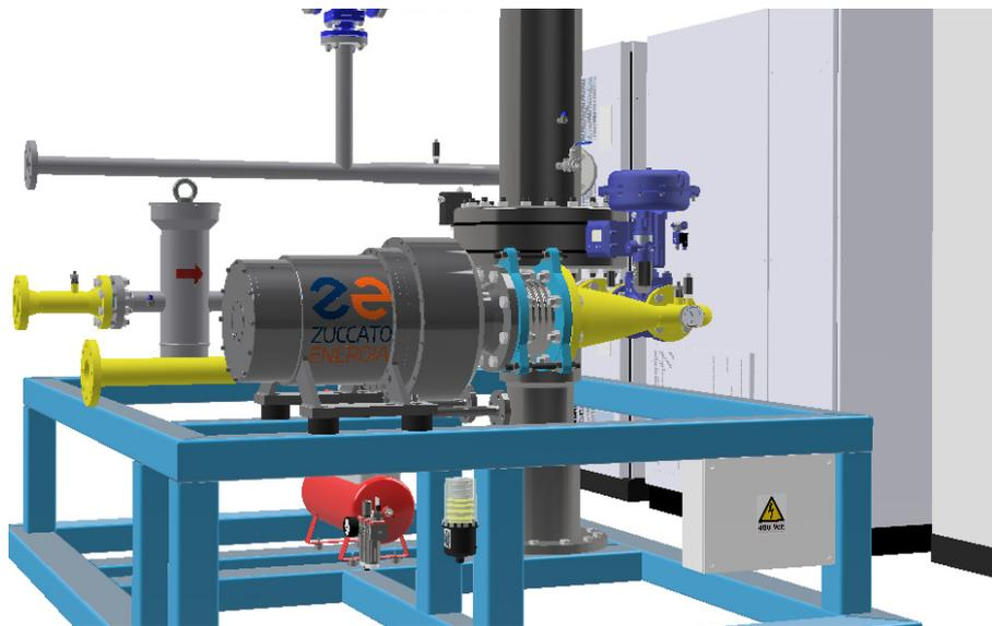
*High speed turbogenerator*
