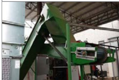
Detail of the conveyor between the chipper and the woodchip yard
