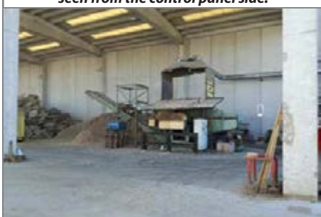
The shredder which reduces the unusable pallets into wooden chips.
