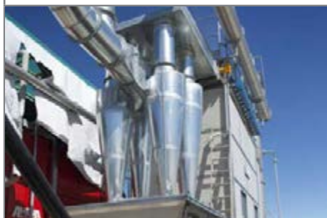
The fuel gas treatment plant with the cover removed To show the filter cyclones
