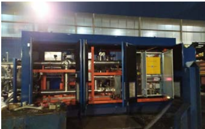
The ORC ZE-200-LT container open for easy maintenance
