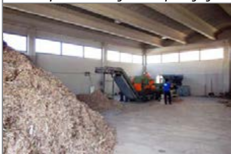
The chipping machine reduces the scraps in fast-burning small wooden chips
