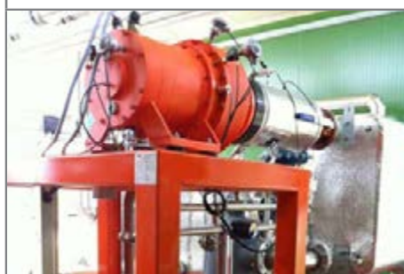
Detail of the 50 kWE turbogenerator
