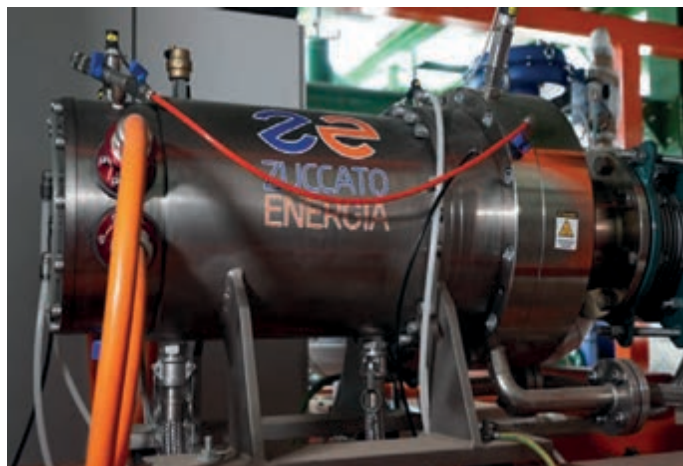
The single stage, radial in-flow turbine directly coupled to the 200kWe generator at the heart of the ORC module
