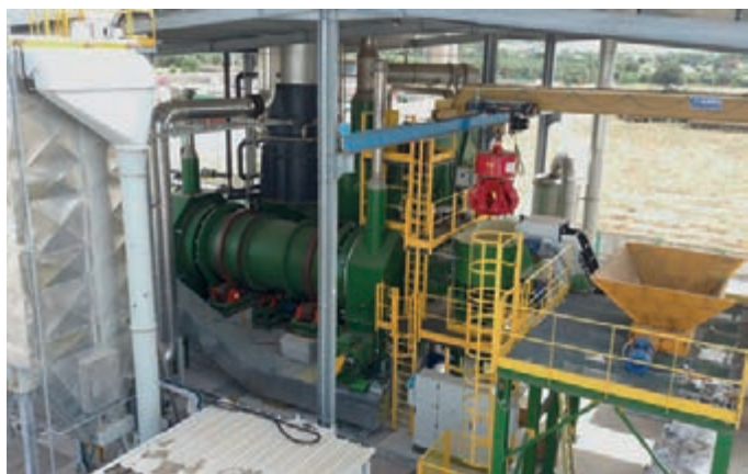
An overall view of rotary kiln (green), syngas boiler (gray), flue gas filter (silver) and waste loading hopper (yellow)
