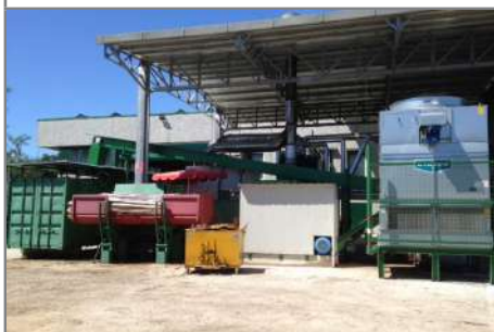
General view from the north side - L to R: woodchip storage (green), wastewood hopper (red), chipper (white), cooling tower (metal).
