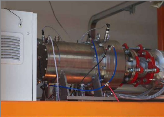
The 150 kWe turbine at the heart of the ZE-150-LT system.
