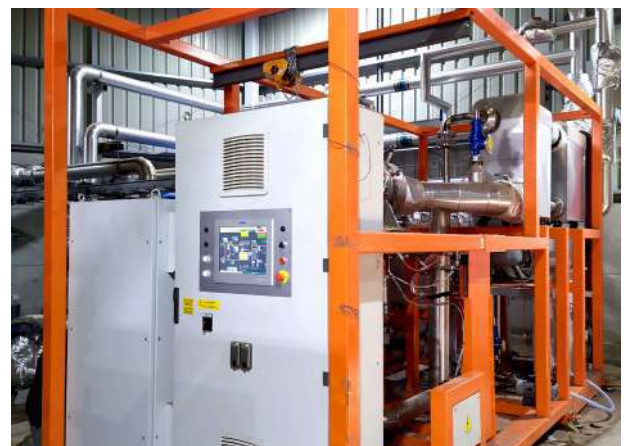
The ZE-105-CHP ORC seen from the control panel side.
