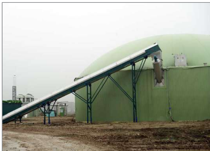
The screw feeding sewage to the fermenters.
