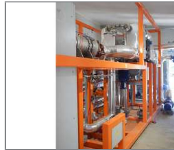
The ZE-175-LT Organic Rankine Cycle energy module, seen from the right side.
