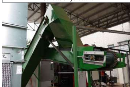
A detail of the conveyor between the chipper and the woodchip storage bin.
