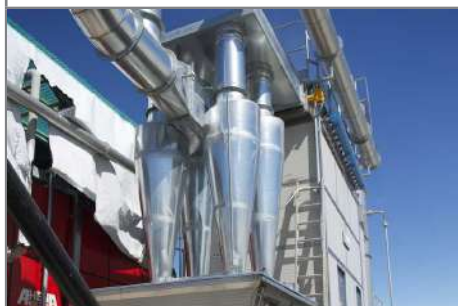
The exhaust treatment system with its cover removed showing the cyclonic filters.
