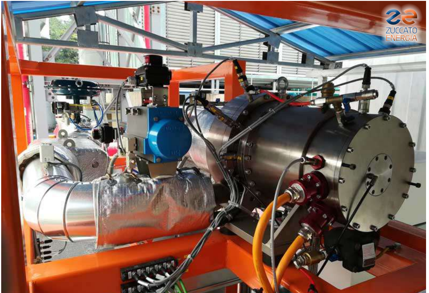
Korea 01 : A detail of the ORC skid - the steel cylinder in the middle is the turbogenerator
